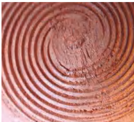
▲ This spiral attempt shows the problem of crumbling short grain on softer timbers
